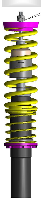
Install the factory top mount and secure it with the supplied nuts. Tightening torque for the piston rod nut is 20 Nm (15 ft-lb). The strut unit has to be installed according to manufacturers instructions settings regarding tightening torque and fixing specifications.
