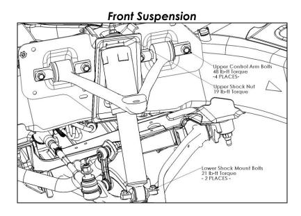
**Caution**: Note the position of any washers between the upper control arm mounts and the frame for use in re-assembly
