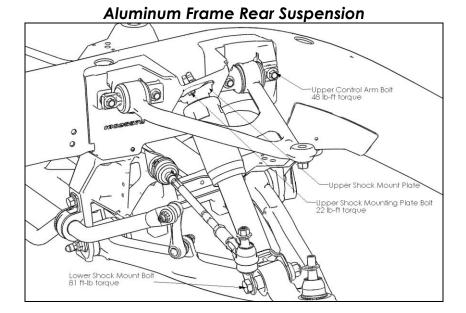
Install the new shock in place. Place the bolt in the lower mount to locate the shock correctly. With the floor jack, raise the lower control arm until the shock is in the correct position. The upper plate mounts with the white dot facing the front of the car. Install the upper mount bolts and torque to 22 lb-ft.
