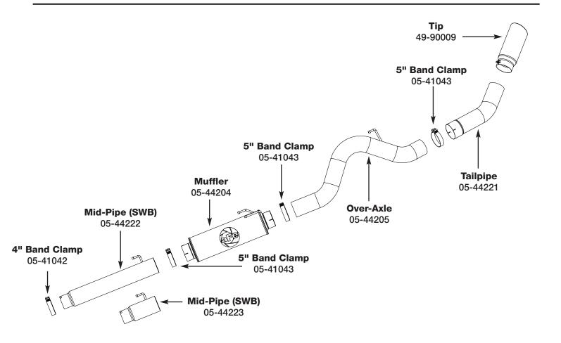
**Step 1:** (Read Instructions prior to installation) Remove your stock exhaust from the rear of your truck working your way forward. It may be necessary to cut the pipes if the slip joints are stuck. Take caution not to damage the factory isolation mounts as they will be reused. It is recommended to not fully tighten the clamps until the entire system has been installed.
