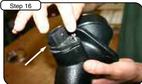
Using provided Gasket and (2) M4x.7x16 screws install MAF Sensor onto aFe intake tube.
