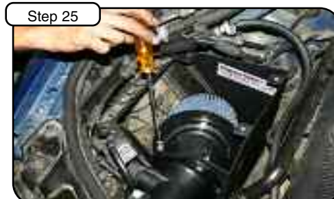
Install high flow aFe air filter. Tighten down clamp using 5/16" Nut driver
