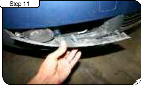
Step 11 Pull off front grill near Passenger side fog lamp.
