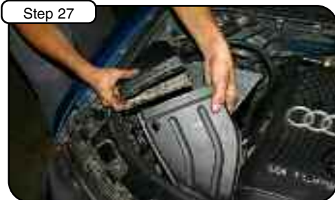
Install factory fresh air duct and tighten down two screws securing it to the core support.
