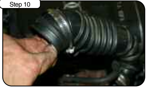
Step 10 Loosen clamp at turbo and Last breather tube. Pull factory tube out of vehicle.
