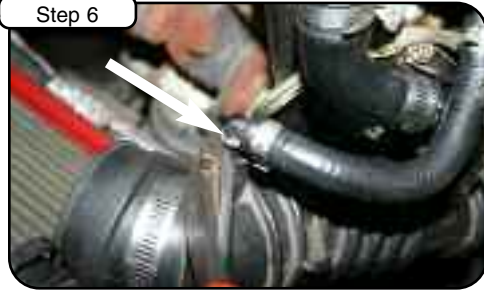
Step 6 Remove clamp holding top breather filter on factory tube.
