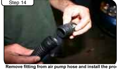
Step 14 Remove fitting from air pump hose and install the provided breather filter. Install the filter onto the air pump and reinstall fog lamp and grill.
