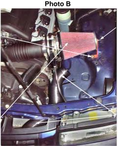
3. Attach the studded lid of the filter to the mounting bracket and secure with a nut and washers supplied.
