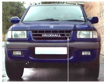
Feed the flexi cold air hose to the front grille. Pierce / drill a 3 mm hole in the plastic sleeve on the hose and secure the hose to the grille using a long plastic tie supplied.
