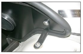
22. Secure the provided bracket (010087) onto the heat shield and inner fender with the provided hardware as shown.
