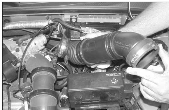
4. Loosen hose clamp at the turbo then remove the intake tube from the vehicle.
