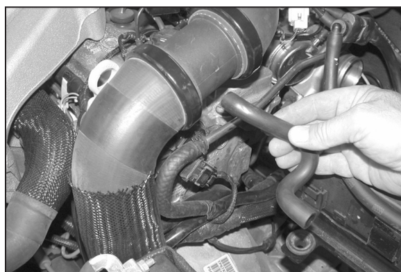
6. Disconnect the crank case vent line from the valve cover as shown.
