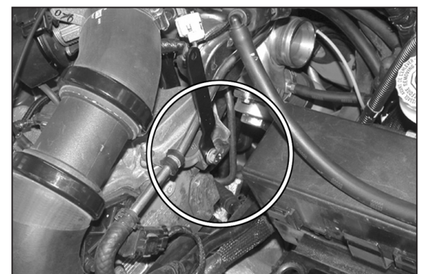
8. Install the new bracket onto the cylinder head with the provided hardware.
