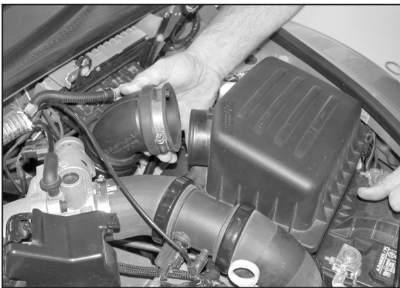
2. Loosen hose clamp at the air box, then remove intake tube from the air box as shown.
