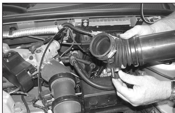
5. Disconnect the vacuum line from the intake tube as shown. NOTE: K&N Engineering, Inc., recommends that customers do not discard factory air intake.
