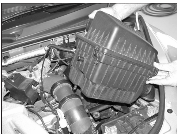
3. Lift firmly up on the air box to remove from car, then disconnect the crank case vent from the air box.
