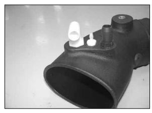
16. Install the provided vent fitting onto the new K&N® intake tube as shown.
