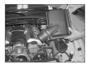
7. Pull up on the air box assembly to dislodge it from the three mounting pins and then remove the air box from the vehicle as shown. **NOTE: K&N Engineering, Inc., recommends that customers do not discard factory air intake.**
