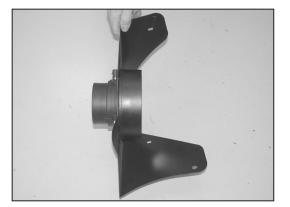
10. Assemble the heat shield and mass air sensor with the provided hardware and gaskets as shown.
