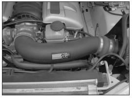
18. Install the K&N<sup>®</sup> intake tube into the silicone hose attached to the throttle body and then onto the mass air sensor. Secure with the provided hose clamps as shown.
