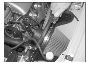
13. Install the heat shield assembly onto the inner fender and start the mount bolts in the air box mounting pin holes, then place the K&N<sup>®</sup> air filter into position. Tighten the heat shield mounting bolts, then install the K&N<sup>®</sup> air filter onto the filter adapter and secure with the provided hose clamp.
