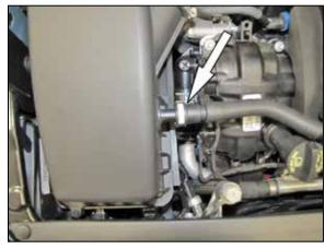
4. Depress the locking tab and then disconnect the crank case vent hose assembly from the air filter housing.
