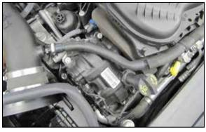
17. Install the crank case quick connect fitting into the factory crank case vent hose and connect it to the fitting installed into the K&N® intake tube.
