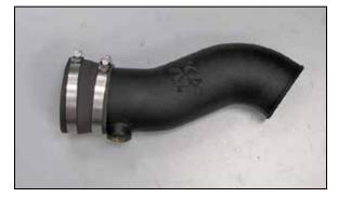
12. Install the provided coupler hose (084091) onto the K&N® intake tube fully but do not tighten at this time.
