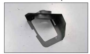
6. Install the provided air filter adapter into the heat shield and secure with the provided hardware.
