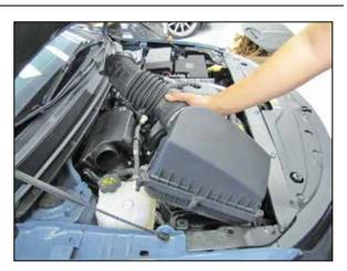
5. Separate the factory intake tube from the intake plenum and then lift up the complete upper air filter housing to dislodge it from the mounting grommets and remove it from the vehicle.
