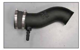
13. Install the provided quick disconnect npt fitting into the K&N® intake tube as shown.
