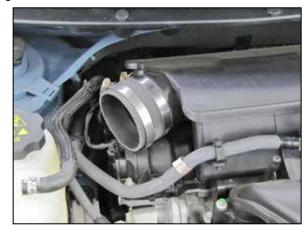
11. Install the provided coupling hose (08690) onto the intake plenum and secure with the provided hose clamp.
