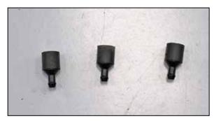
7. Install the three provided heat shield mounting studs onto the rubber mounted studs as shown.
