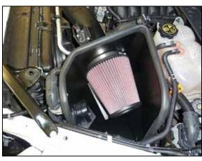
27. Install the K&N® air filter onto the adapter and secure with the provided hose clamp.
