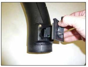
22. Install the mass air sensor into the K&N® intake tube and secure with the provided hardware.
