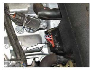
33. Reconnect the mass air sensor electrical connection.
