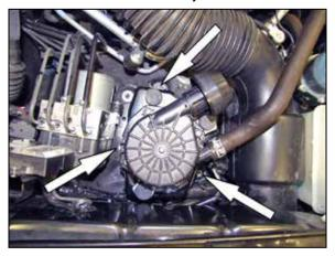
4. Remove the three bolts securing the secondary air pump and then disconnect the electrical connection and remove the secondary air pump from the engine compartment.
