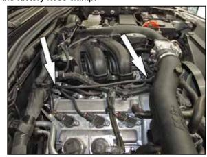
32. Connect the provided fuel pressure vent hose to the fuel pressure regulator and then connect the open end to the fitting installed into the K&N® intake tube.
