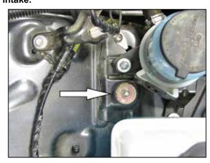
11. Install the provided 8mm rubber mounted stud into the intake resonator mounting location as shown.
