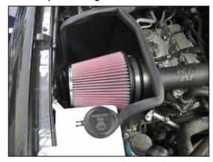
37. Install the K&N® air filter and secure with the provided hose clamp.
