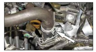
3. Release the spring clamp securing the secondary air hose to the union on the engine and then disconnect the secondary air hose.
