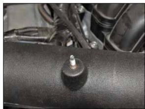
35. Install the engine cover mounting stud into the  $K\&N^{\tiny @}$  intake tube.
