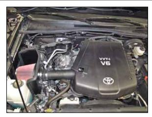
38. Reconnect the vehicle's negative battery cable. Double check to make sure everything is tight and properly positioned before starting the vehicle.
