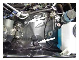
12. Install the two remaining 6mm rubber mounted studs into the secondary air injection pump mounting locations.
