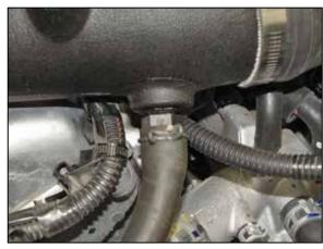
31. Connect the crank case vent hose to the fitting installed into the K&N<sup>®</sup> intake tube and secure with the factory hose clamp.
