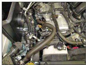
21. Install the secondary air pump onto the brackets previously installed and secure with the provided hardware. Reconnect the secondary air hose to the fitting and secure with the factory spring clamp.
