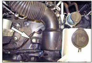
6. Remove the two bolts securing the intake resonator to the inner fender and then remove the intake tube/resonator assembly from the engine compartment.
