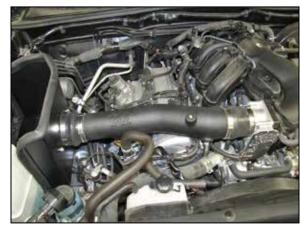
**3**0. Install the K&N® intake tube into the silicone hose at the filter adapter far enough to gain clearance into the silicone hose at the throttle body, then install the tube into the throttle body silicone hose and secure with the provided hose clamps. **NOTE: Do not completely tighten at this time.**
