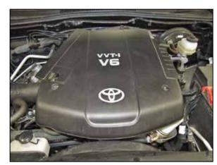
36. Install the engine cover and secure with the factory retaining nuts.
