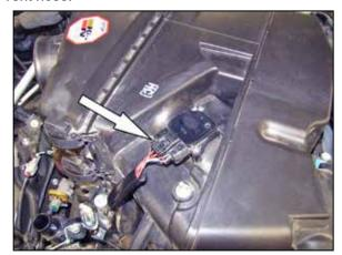
9. Disconnect the mass air sensor electrical connection and unhook the wiring harness from the air filter housing.
