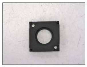
26. Install the provided gasket onto the mass air sensor adapter.
