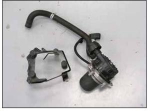
20. Separate the secondary air pump motor from the mounting bracket.
