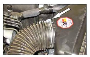
5. Loosen the hose clamp securing the intake tube to air filter housing.
