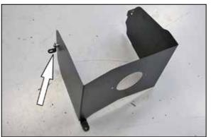
8. Install the heat shield mounting bracket (070066) onto the heat shield using the provided spacer and hardware.
