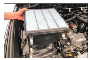
7. Loosen the three bolts securing the lower air box and then remove the lower air box from the vehicle. NOTE: K&N Engineering, Inc., recommends that customers do not discard factory air intake.
