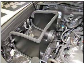
13. Set the heat shield into the engine compartment and secure with the provided hardware.
