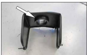
11. Install the filter adapter onto the heat shield and secure with the provided hardware.
