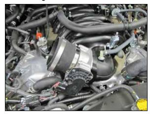
14. Install the coupler hose (08050) onto the throttle body and secure with the provided hose clamp.
