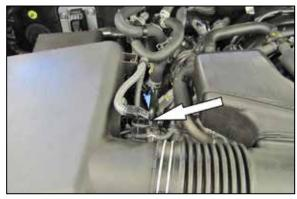
2. Disconnect the mass air sensor electrical connection and then unhook the wiring harness from the air box.
