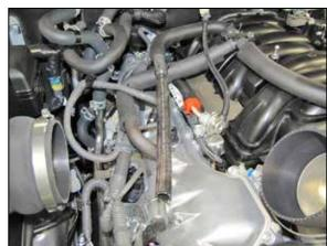
22. Install the crank case vent hose assembly into the factory crank case vent hose as shown.
