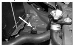
14. Install the provided rubber mounted stud into the threaded hole where the factory airbox was mounted.
