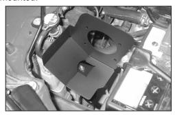
15. Place the heat shield onto the rubber mounted stud, then place the provided hardware. Pivot the heat shield around.
