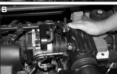
7. Loosen the hose clamp at the throttle body.
