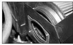
20. Place the gasket on the heat shield, as shown.
