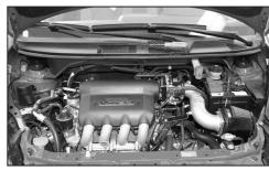
25. Check for best fit, then tighten all hardware and hose clamps.
