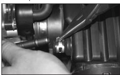
3. With pliers, depress the hose clamp and remove the crankcase vent (CCV) hose.
