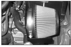
16. Place the filter assembly on the heat shield as shown. Tighten the lock nut on the vibration mount. NOTE: Heat shield should be perpendicular (90 degrees) to the battery. It may be necessary to loosen the battery and move it back to gain clearance for the heat shield
