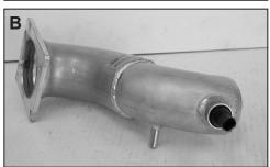
10. Push the provided grommet into the air temp. sensor vent tube on the  $K\&N^{\otimes}$  intake tube. Then install the air temp sensor into the grommet.
