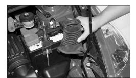
5. Separate the fresh air duct from the factory intake and completely remove.
