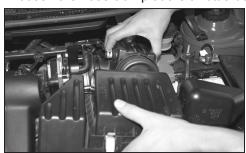
8. Remove the factory airbox by pulling away from the throttle body and lifting upwards.
