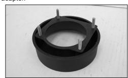
12. Install the gasket onto the filter adaptor as shown.
