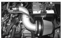
21. Install the K&N® intake tube on the heat shield first, then to the hose on the throttle body.
