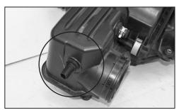
9. Remove the air temperature sensor from the factory airbox.
