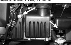
6. Loosen and remove the 2 bolts that secure the factory airbox to the vehicle.
