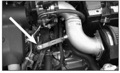
23. Install the "L" bracket and secure with the provided hardware.
