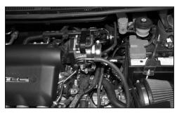
18. Attach the silicone hose to the crankcase vent hose on the engine valve cover as shown.
