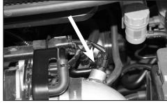
24. Clip the ATS harness into the air temperature sensor.
