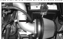
22. Secure the K&N® intake tube to the heat shield using the provided hardware.
