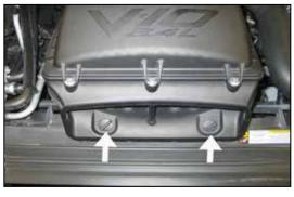
4. Unscrew and remove the two air box fastener nuts shown.
