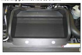
Install the heat shield onto the air box mounting location and secure with the provided hardware.
