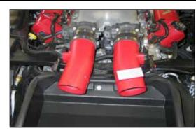
18. Install the right side K&N® intake tube into the silicone hose at the throttle body and then secure the tube to the mounting bracket with the provided hardware.
