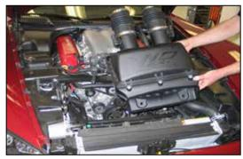
6. Dislodge the air box assembly from the mounting grommet and remove the air box from the vehicle.
