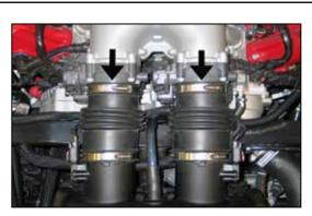
3. Loosen the two hose clamps which secure the stock intake tubes to the throttle bodies.
