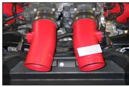
19. Align the intake tubes so that they are straight and even coming out of the throttle bodies, then tighten the heat shield mounting bolts and tube mounting bolts.
