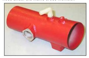
14. Install the 90° vent fitting into the left side K&N<sup>®</sup> intake tube as shown.
