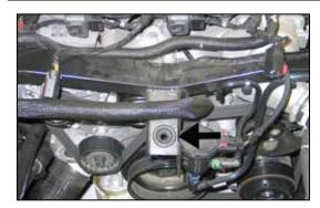
7. Remove the rubber mounting grommet shown.
