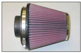
20. Install the filter adapters into the K&N® air filters and secure with the provided hose clamps.
