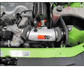
16. Install the K&N® intake tube assembly into position, Slide the coupling hoses out and onto the throttle body and filter adapter. Then adjust the tube and hoses for proper fit and secure with the provided hose clamps.
