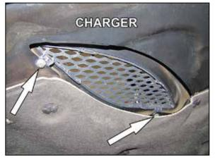
20. If the vehicle is to be driven during inclement or wet weather it is recommended the shield be installed onto the hood vent to guard the air filter from concentrated water. Remove the two bolts that secure the factory vent grid.
