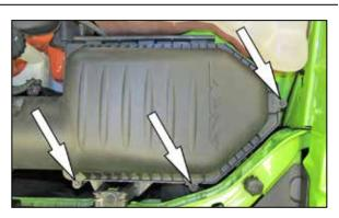
filter housing and then remove the upper air filter housing and intake tube.
