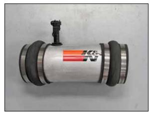
15. Install both of the coupling hoses (08418) onto the  $K\&N^{\otimes}$  intake tube as shown.
