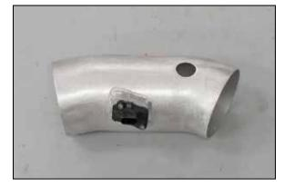
13. Install the mass air sensor into the K&N<sup>®</sup> intake tube and secure with the provided hardware.
