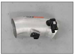
14. Install the provided grommet and pressure sensor/vent assembly into the K&N $^{\odot}$  intake tube as shown.
