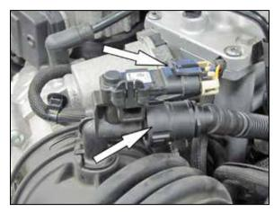
3. Disconnect the pressure sensor electrical connection and disconnect the crank case vent hose from the fitting.
