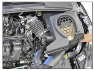
2. Lift off the engine cover and remove it from the vehicle.
