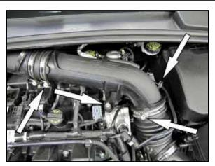
3. Remove the bolt securing the factory intake tube to the engine shown. Next loosen the hose clamps and unhook the vent line from the intake tube and remove the intake tube from the vehicle.
