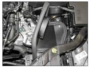
13. Install the heat shield assembly into the vehicle so the mounting studs insert into the grommets.
