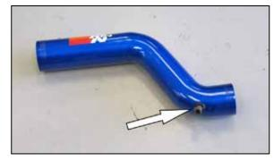
15. Install the grommet provided and the factory inlet air temperature sensor into the K&N<sup>®</sup> intake tube as shown.
