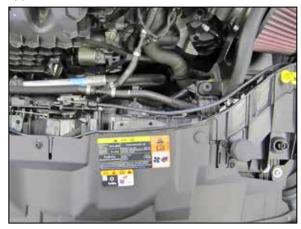
21. Using the K&N<sup>®</sup> Fresh air duct as a guide, mark the two hole locations onto the fresh air duct in the core support. Next remove the K&N<sup>®</sup> fresh air duct and drill two  $\frac{1}{4}$ "id holes into the factory fresh air duct in the core support at the marked locations.
