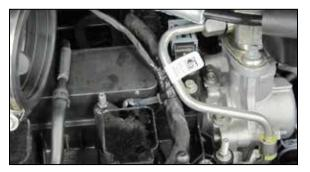
16. Unhook the wiring harness clip from the mounting stud, route the harness next to the coil and fuel line and secure the harness to the fuel line with the provided tie wrap.
