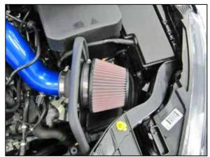
19. Install the K&N<sup>®</sup> air filter onto the filter adapter and secure with the provided hose clamp. NOTE: Drycharger<sup>®</sup> air filter wrap; part # RU-5163DK is available to purchase separately. To learn more about Drycharger<sup>®</sup> filter wraps or look up color availability please visit http://www.knfilters.com<sup>®</sup>.
