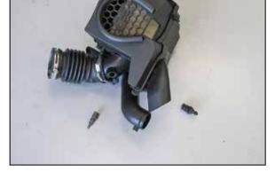
11. Remove the inlet air temperature sensor and mounting post from the factory air box.
