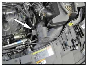
5. Release the inlet air duct from the air box.
