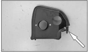
12. Install the mounting post from the previous step onto the  $K\&N^{\mbox{\tiny \ensuremath{\$}}}$  heat shield as shown.
