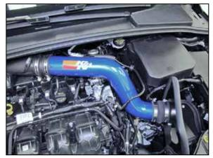
17. Install the K&N<sup>®</sup> intake tube into the factory coupler and then into the K&N<sup>®</sup> coupler, adjust the tube for best fit and then secure with the provided hose clamps.
