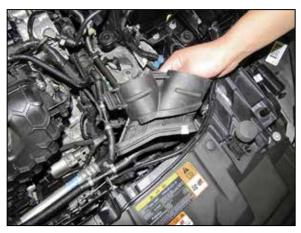
7. Remove the inlet air duct from the core support.
