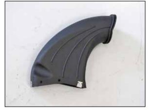
23. Install the two clips from the previous step onto the K&N $^{\circ}$  fresh air duct in the same position as the factory.
