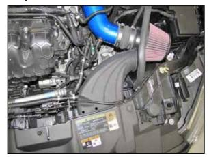
24. Install the K&N<sup>®</sup> fresh air duct into the heat shield and core support as shown and secure with the two provided retaining clips.
