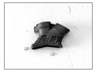
22. Remove the two clips from the factory inlet air hose.
