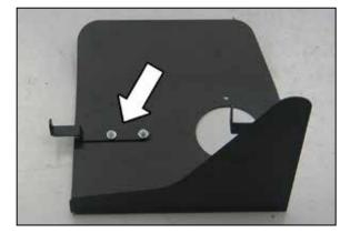
9. Install the heat shield mounting bracket (083126A) onto the heat shield and secure with the provided hardware.
