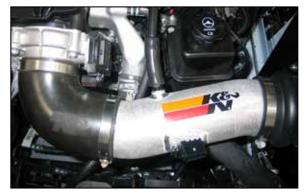
20. Remove the 90° vent hose from the crank case vent tube. Then install the provided silicone vent hose; trim the hose for proper fit and install it onto the fitting installed into the K&N<sup>®</sup> intake tube.
