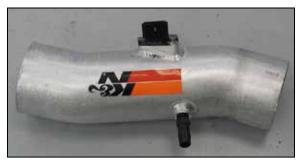
18. Install the provided vent fitting into the  $K\&N^{\otimes}$  intake tube as shown.
