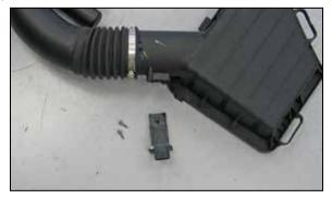
16. Remove the two screws that secure the mass air sensor into the factory intake tube and then remove the mass air sensor from the factory upper air box.
