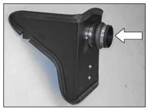
13. Install the provided silicone hose (5-576) onto the filter adapter as shown and secure with the provided hose clamp.
