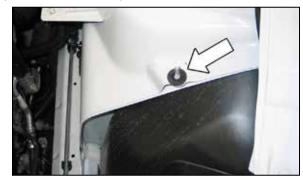
14. Install the provided rubber fender washer onto the outer air box mounting stud.
