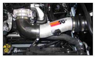
19. Install the provided silicone hose (08629) onto the K&N<sup>®</sup> intake tube as shown. Install the K&N<sup>®</sup> intake tube assembly onto the throttle body and filter adapter, adjust the tube in the hoses for proper fitment. Once properly fitted, secure the tube with the provided hose clamps.
