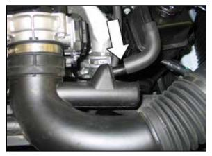
4. Disconnect the crank case vent hose from the stock intake tube.
