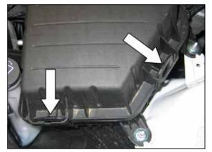
6. Unlatch the upper air box clips and then remove the upper air box and intake tube assembly.
