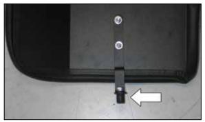
12. Install the provided inserted nut onto the heat shield mounting bracket and secure with the provided hardware.
