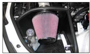
21. Install the K&N<sup>®</sup> air filter and secure with the provided hose clamp.
