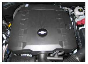
2. Remove the oil fill cap and then lift up and remove the engine cover. Reinstall the oil cap.
