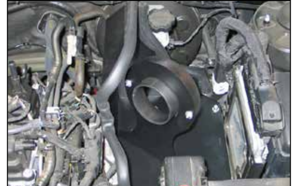
21. Set the heat shield assembly onto the rubber mounted studs and secure with the provided hardware.
