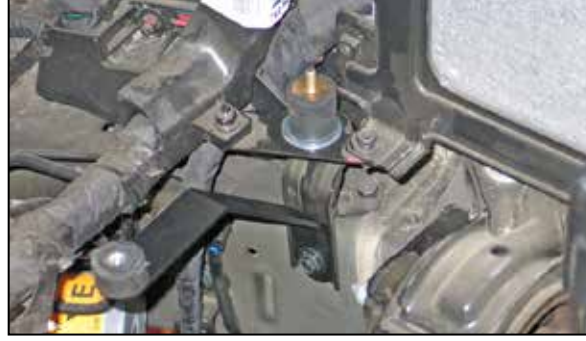
14. Install the provided large rubber mounted stud onto the airbox mounting grommet location using the provided hardware.
