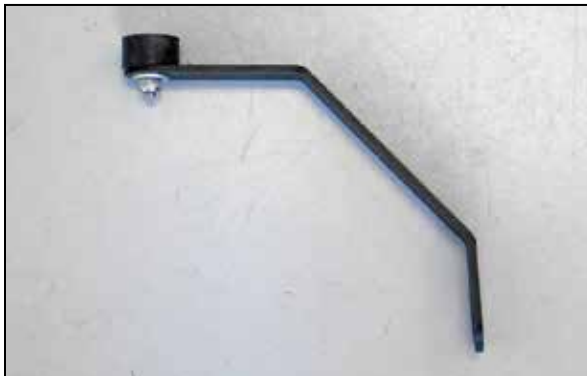
12. Install one of the provided rubber mounted studs onto the heat shield mounting bracket as shown using the provided hardware.
