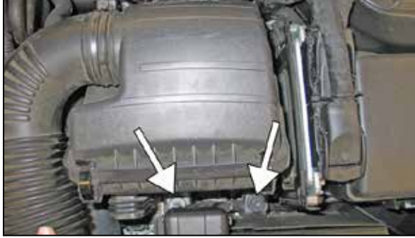
8. Remove the two bolts that secure the airbox.
