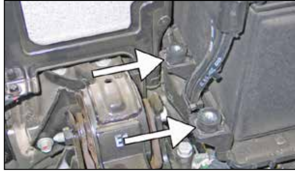
15. Install the two remaining rubber mounted studs onto the airbox mounting locations as shown.
