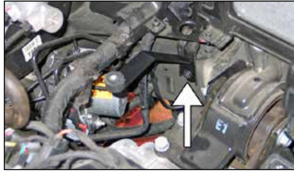
13. Install the heat shield mounting bracket assembly onto the airbox mounting bracket and secure using the provided hardware.
