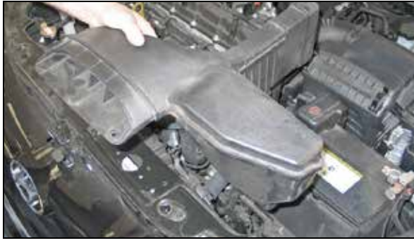
7. Remove the fresh air duct from the vehicle.
