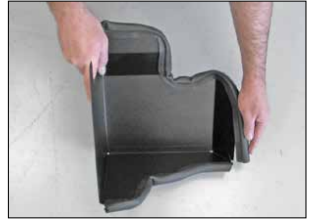
18. Install the longer 25" section onto the heat shield as shown.
