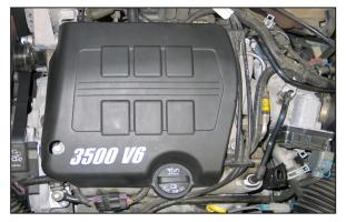
3. Remove the oil filler cap. Pull up firmly on the engine cover, removing it from the vehicle.
