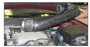
7. Remove the stock intake tube from the vehicle.
