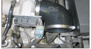
14. Install the provided silicone hose (08629) onto the throttle body with the provided hose clamp.
