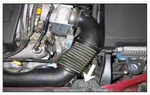
6. Loosen the hose clamp that secures the stock intake tube to the throttle body. Remove the bolt that secures the stock intake tube to the core support.
