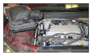
10. Remove the stock air box from the vehicle. NOTE: K&N Engineering, Inc., recommends that customers do not discard factory air intake.
