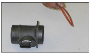
13. Remove the O-ring from the mass air sensor.
