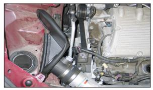
24. Install the mass air sensor and heat shield assembly. Secure with the provided hose clamp as shown.
