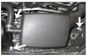
9. Remove the three bolts that secure the stock air box. On vehicles equipped with air injection, release the retaining clips and unhook the air injection hose from the air box lid. **NOTE: The bolt that secures the A/C line to the factory air box will be re-used.**
