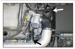
25. Cut the end of the crank case vent line, then install the provided silicone vent line onto the stock vent line and then onto the K&N<sup>®</sup> Intake Tube as shown.
