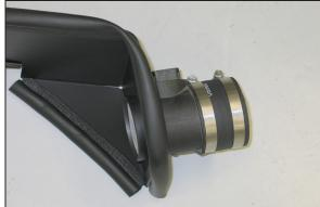
18. Install silicone hose (#08690) onto the mass air sensor with the provided hose clamp as shown.
