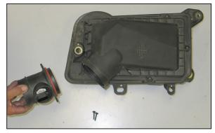
12. Remove the two Torx screws that secure the mass air sensor to the stock air box.
