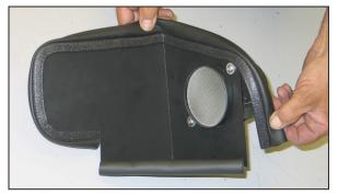
17. Install the provided edge trim (long) onto the heat shield as shown.
