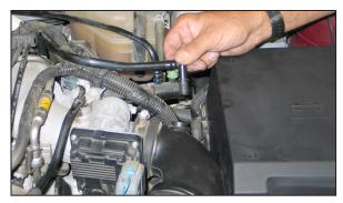
4. Remove the crank case vent tube from the stock intake tube.
