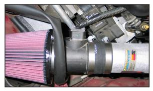
28. Re-connect the mass air sensor as shown. NOTE: Due to Manufacturer tolerances, it may be necessary to unclip the wiring harness and adjust it for more slack.
