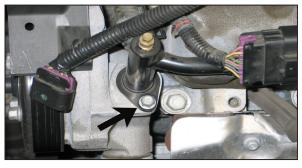
20. On vehicles equipped with the above style heater hose tube, remove the mounting bolt shown. **NOTE: The bolt will be re-used.**
