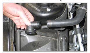
10a. On vehicles equipped with air injection, cut the clamp which secures the elbow fitting to the hose and then remove the elbow fitting from the hose.
