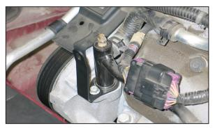
21. Install the correct tube mounting bracket (06496 or 070049) to match the style heater hose tube as shown in the above photos and secure with the factory bolt removed in step #20a. **NOTE: on vehicles equipped with a vibration dampening shock on the passenger side engine mount, be sure to place the spacer between the mounting bracket and engine. Do not completely tighten at this time.**
