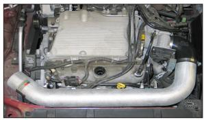
22. Install the K&N<sup>®</sup> Intake Tube into the silicone hose at the throttle body and align the intake tube with the mounting brackets installed in the previous step. Secure the intake tube with the provided hardware and hose clamp.
