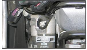
20a. On vehicles equipped with the above style heater hose tube, remove the mounting bolt shown. **NOTE: This bolt will be reused in a later step**
