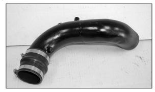
22. Install the hump hose onto the K&N<sup>®</sup> intake tube with the hose clamps provided.
