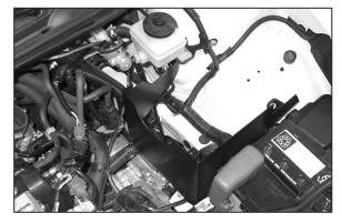
15. Using the provided hardware fasten the heat shield to the threaded hole on the strut tower.
