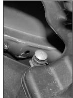
11. Remove the air inlet duct retaining screws from the inner fender as shown.
