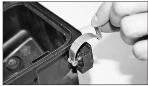
25. Remove the two retaining clips from the lower air cleaner by pushing down as shown.
