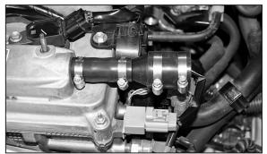
19. Connect the crankcase vent assembly to the vent fitting on the valve cover.
