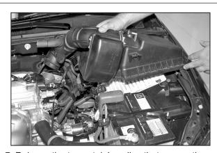
7. Release the two retaining clips that secure the air cleaner cover. Depress the spring clamp on the stock intake tube at the throttle body, then, remove the complete upper air intake assembly as shown.
