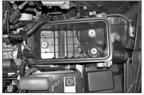
8. Loosen and remove the three bolts that retain the lower air cleaner as shown.
