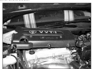
2. Remove the engine cover, which is secured by two acorn nuts as shown.
