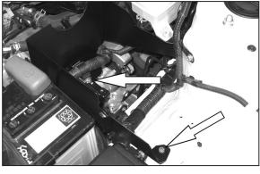
16. Using the bolt removed in step 13, fasten the heat shield & wire harness bracket, then resecure bolt. With the provided hardware secure the heat shield to the factory air cleaner mounting point located on the inner fender apron.
