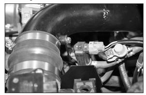
31. Fasten the vacuum switching valve assembly to the threaded boss on the K&N® intake tube, using the provided hardware.
