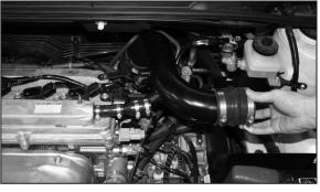
23. Install the K&N® intake tube inserting it into the tapered hose at the throttle body.
