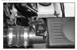
33. Reconnect the mass air sensor electrical connection. Check everything for best fit and clearance then tighten all hardware and hose clamps.
