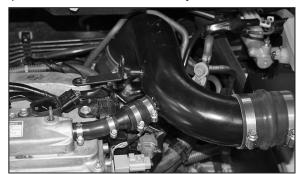
24. Connect the crankcase vent assembly to the vent fitting on the K&N $^{\! \otimes}$  intake tube and tighten all hose clamps.
