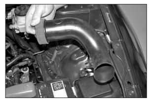
10. Remove the air inlet duct by rotating it counter clockwise as shown.
