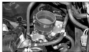
20. Using the hose clamps provided, install the tapered hose with clamps onto the throttle body as shown.
