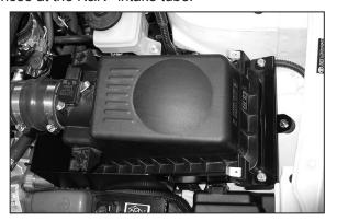
29. Using the provided hardware, fasten the filter assembly mounting bracket to the threaded inserts in the filter cage, then to the rubber mounted stud located on the inner fender apron.
