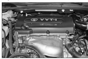
34. Reinstall the engine cover and acorn nuts that were removed in step #2 as shown.
