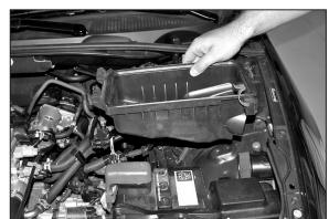
9. Remove the lower air cleaner assembly as shown.
