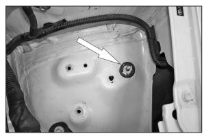
14. Install the rubber mounted stud provided into the threaded hole in the inner fender apron as shown.
