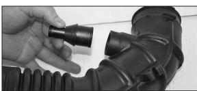
17. Disassemble the crankcase vent hose, union tube and stock intake tube as shown.
