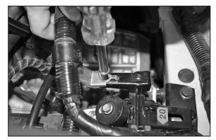
13. Remove the bolt that retains the wire harness bracket to the transmission mount.
