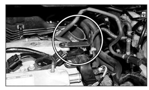
21. Using the hardware provided, attach the "L" bracket to the threaded hole located on the rear portion of the valve cover as shown.
