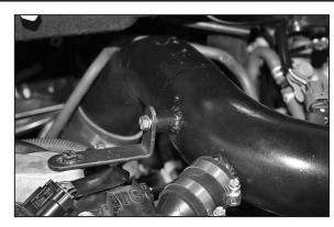
32. Using the hardware provided, fasten the "L" bracket to the threaded boss on the K&N® intake tube as shown.
