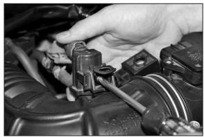
5. Detach the vacuum switching valve from the stock intake tube.
