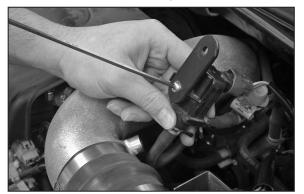
30. Attach the flat bracket to the vaccum switching valve using the a buttonhead screw.
