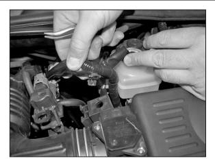
4. Detach the wire harness from the air cleaner assembly as shown.
