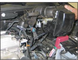
9. Release the spring clamp that secures the stock intake tube at the throttle body. Then, remove the complete intake tube assembly as shown.
