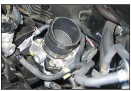
18. Install silicone hose (#084016) onto the throttle body and secure with the provided hose clamp.
