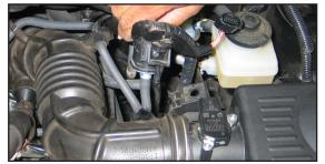
4. Un-hook the EVAP solenoid valve from the stock intake tube as shown.
