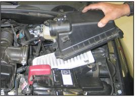
6. Un-hook the upper air box mounting clips, then remove the upper air box as shown.
