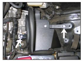
15. Set the heat shield into position as shown. Then, secure the heat shield brackets using the provided hardware as shown.
