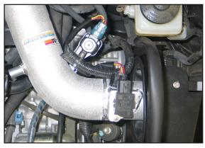
23. Secure the EVAP mounting bracket to the intake tube with the provided hardware.
