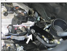
19. Install intake tube mounting bracket (#26661) onto the cylinder head and secure with the provided hardware as shown.
