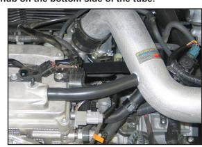
24. Install the provided crank case vent hose as shown.
