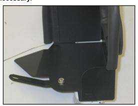
13. Install heat shield mounting bracket (#26662) onto the heat shield using the provided hardware as shown.
