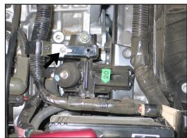
10. Remove the bolt that secures the wiring harness as shown.
