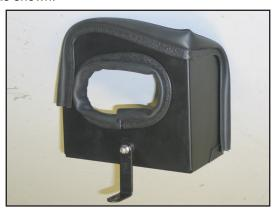
14. Install heat shield mounting bracket (#07093) onto the heat shield using the provided hardware as shown.
