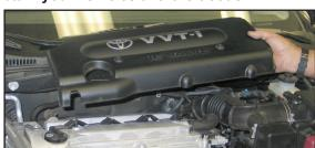
2. Remove the two nuts that secure the engine cover. Remove the engine cover from the engine.
