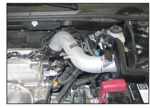
22. Install the K&N® intake tube into the silicone hose at the throttle body and align with the mounting bracket. Secure the intake tube with the provided hardware and hose clamp as shown.
