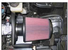
25. Install the K&N® air filter onto the K&N® intake tube and secure with the provided hose clamp. NOTE: Drycharger® air filter wrap; part # RX-4730DK is available to purchase separately. To learn more about Drycharger® filter wraps or look up color availability please visit http://www.knfilters.com®.
