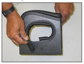
12. Install the short edge trim onto the heat shield as shown.
