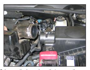
5. Loosen the hose clamp that secures the intake tube to the upper air box, then disconnect the intake tube as shown.
