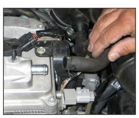
8. Un-hook the crank case vent hose from the valve cover as shown.
