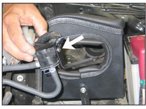
21. Secure the provided bracket (#070622) to the EVAP solenoid valve as shown.
