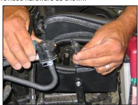
20. Remove the screw that secures the mounting bracket to the EVAP valve, then remove the mounting bracket as shown.
