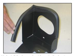
11. Install the long edge trim onto the heat shield as shown.
