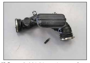
27. Remove the inlet air temperature sensor from the factory intake plenum as shown. NOTE: Use caution working with the inlet air
