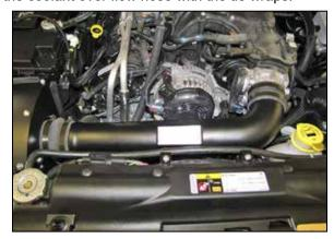
31. Install the K&N® intake tube into the silicone hose at the filter adapter and then into the hose at the throttle body, then secure with the provided hose clamps.
