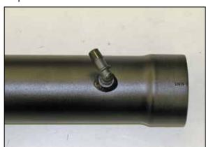
25. Install the 90°, ½" vent fitting into the K&N® intake tube as shown.
