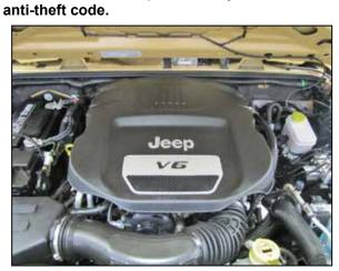
2. Lift up and remove the engine cover.
