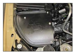
22. Install the K&N® filter lid and secure with the provided hardware.
