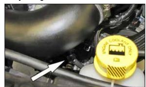
33. Reconnect the inlet air temperature sensor electrical connection and then reinstall the engine cover.
