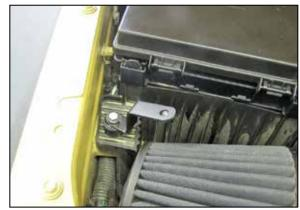
21. Install the provided bracket (083163) onto the rubber mounted stud using the provided hardware.
