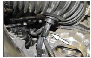
6. Lift up the intake tube and then disconnect the inlet air temperature electrical connection. Then remove the intake tube from the vehicle.
