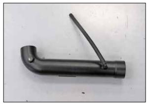
26. Install the provided crank case vent hose onto the fitting as shown.
