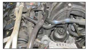
32. Connect the open end of the crank case vent hose to the factory crank case vent tube as shown. NOTE: the use of "WD-40" or similar lubricant may be helpful in installing the hose onto the factory tubing.
