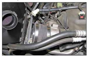
16. Install the provided step coupler (08497) onto the throttle body and secure with the provided hose clamps.
