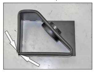
8. Install the provided edge trim onto the K&N® heat shield as shown.
