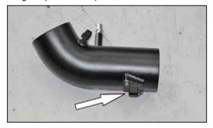
14. Install the humidity sensor into the K&N® intake tube and secure with the provided hardware.
