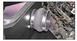
15. Install the provided coupler hump hose (08418) onto filter adapter and secure with the provided hose clamp.
