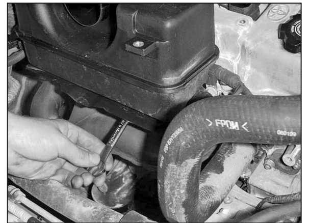
5. Loosen and remove the two nuts that secure the resonator.
