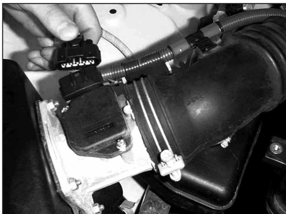
2. Disconnect the mass air sensor electrical connection.
