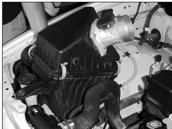
4. Loosen the three bolts that secure the air cleaner assembly, then remove the complete assembly as shown.
