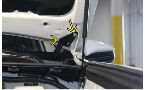
2. Install the driver's side bracket by hand tightening the provided washer and M8 bolt. Angle the bracket to give clearance to the rear hood hinge bolt for removal.
