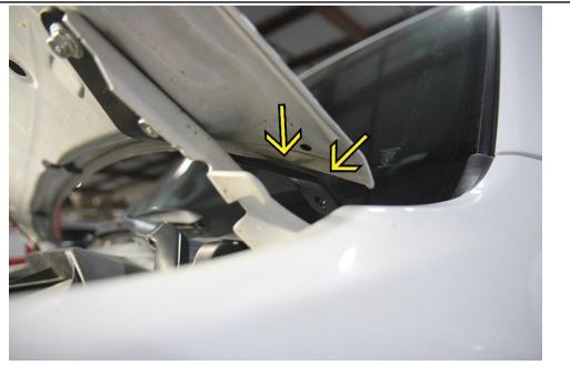
4. Before tightening the bolts, check for clearance between the hood and the ditch light bracket. Adjust the bracket accordingly and make sure to realign the hood to its original position.
