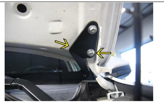
3. Remove the rear bolt from the hood hinge in order to rotate the bracket to line up the rear hood hinge mounting hole and rear bracket mounting hole. Install and hand tighten the provided washer and M8 bolt.
