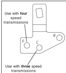
Leave the swivel out of the hole and move the selector lever to Park, all the way forward. Also move the shifter to Park position. (See operation section, page 8). Reinsert the swivel into the hole in the selector lever. Check to see that the swivel will slide freely in and out of the hole in the selector lever in this position. If it does not slip in freely, adjust the swivel slightly until it will slip into the hole in the lever.
