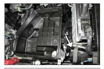
k. Disconnect lower airbox from inlet tube. Remove the lower airbox and set aside.
