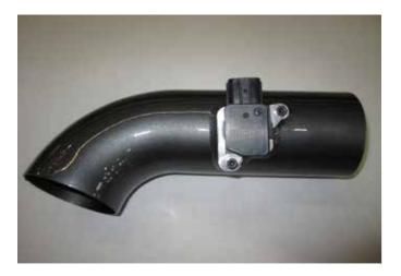
b. Install the MAF sensor onto the lower intake tube (K) using the provided M4 bolts (M), Tighten with an allen wrench.
