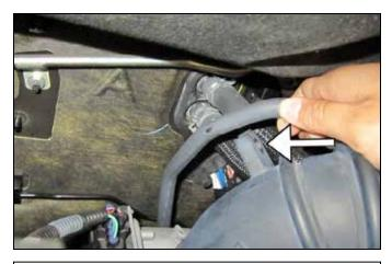
f. Unclip the VSV hose on the rear side of the inlet tube. Tuck the hose and VSV away from inlet tube.
