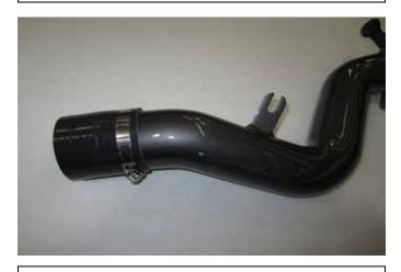
e. Slide coupler (L) onto the upper tube about 1-1/8th inch and fasten with #44 hose clamp (H)
