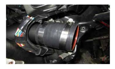
n. slide the additional #48 hose clamp (I) onto the coupler (L) .
