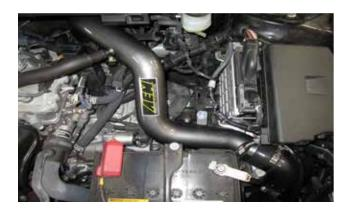
u. AEM® intake system installed.
