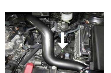
j. Position intake pipe (A) so the mounting bracket slides into position over the rubber mount, then loosely fasten with the provided washer (F) and M6 nut (G). Tighten the hose clamp to secure the intake tube to the throttle body.
