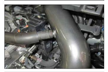
k. Connect the valve cover hose to the intake tube and secure with the stock spring clamp.
