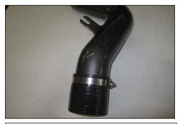
h, Install coupler (L) and hose clamp (H) on the upper intake tube.
