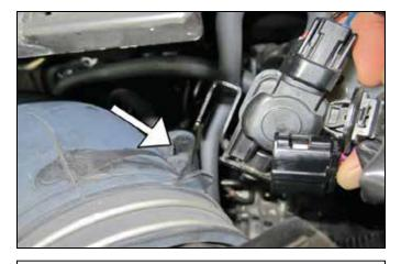
e. Unhook the vacuum switching valve (VSV) from the rubber inlet tube bracket.
