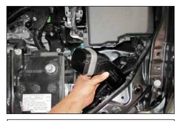
I. Slide the inlet tube down towards the headlight slightly and remove the inlet tube from the vehicle.
