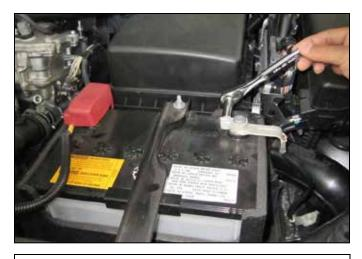
b. Disconnect negative terminal on battery using 10mm socket and tuck away from battery.
