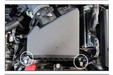
h. Locate the two clips securing the airbox lid next to the battery. Unhook the clips and slowly remove the airbox lid and tube assembly, ensuring the MAF wire harness, VSV, and VSV hose are not snagged during removal.
