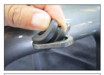
c. Insert the rubber grommet (D) into the VSV bracket as shown.
