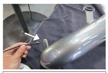
d. Insert the tree mount zip tie (C) into the bracket of the upper intake tube as shown.
