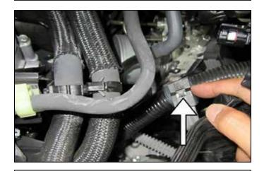
j. Detach the wire harness from the rear side of the lower airbox and slide off the metal bracket by slightly pulling back on plastic tab.
