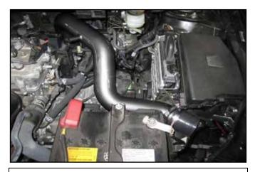
i. Maneuver the inlet side of the upper intake tube through the channel near the battery and under the wire harness. Pull back the plastic cover panel slightly and carefully slide the outlet side of tube towards throttle body. Insert the #48 hose clamp (I) over the coupler/ throttle body.
