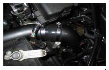
r. Attach the lower intake pipe (K) to the coupler and maneuver the intake pipe so the bracket slides into place. Check for clearance on the headlight housing and fog light housing (if applicable). Tighten all clamps and nuts once proper clearance is obtained.
