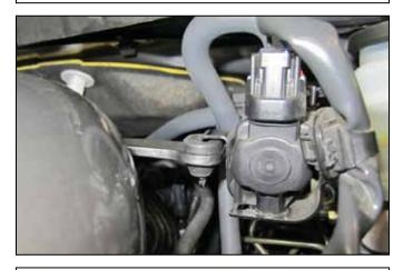
I. Slide the VSV bracket into the rubber grommet as shown.
