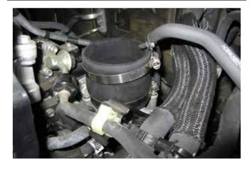
g. Install the reducer coupler (b) on to the throttle body using hose clamps (h) and (l).
