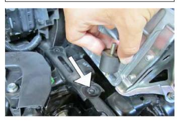
f. Install the set screw in the female side of the rubber mount with 3/8" left out. Then thread it into the location shown in the picture.
