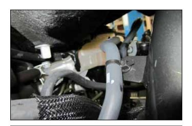
m. Fasten the VSV hose to the upper intake pipe using the provided tree mount zip tie, trim off excess.
