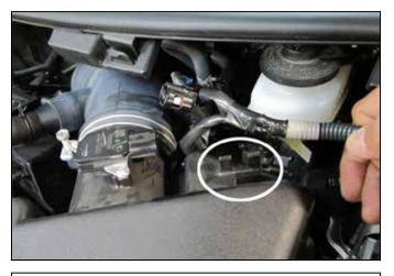
c. Disconnect wire harness from MAF sensor and unclip MAF wire harness from stock airbox.
