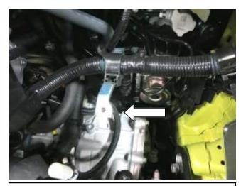
h. Remove the M6 bolt that secures the wiring harness to the lower air box and remove the lower air box.
