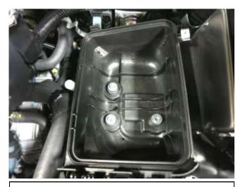
g. Remove the three M6 bolts that secure the lower air box to the engine compartment.
