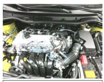
b. Remove the engine cover by gently pulling it up from the engine.
