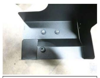
b. Install the grommets and metal sleeves onto the AEM heat shield as shown.
