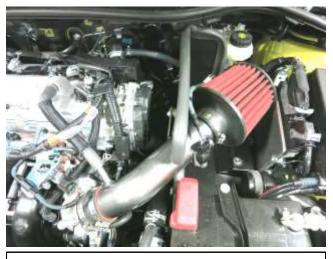
I. Reconnect the vent hose to the intake tube and tighten all hose clamps .
