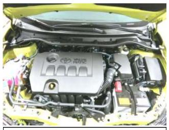
a. 2016 Scion iM with factory air intake system.
