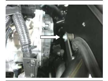
i. Secure the AEM intake tube to the rubber mounted stud with the supplied M6 nut and washer.
