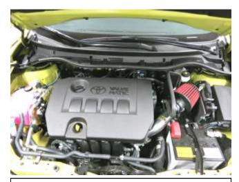
n. AEM 21-776C intake system installed.
