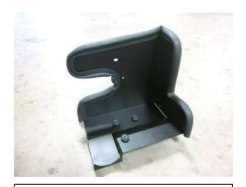
c. Install the supplied rubber edge trim on the AEM heat shield as shown.
