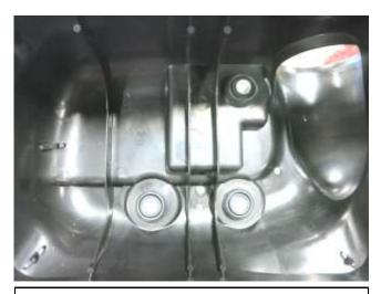
a. Remove the three rubber grommets and metal sleeves from the lower air box.
