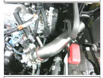
h. Install the complete intake tube assembly to the coupler and line up bracket with the rubber mounted stud.
