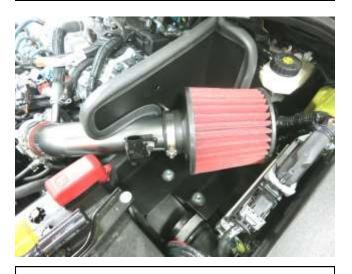
j. Install the AEM filter onto the intake tube as shown.
