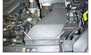
2. Remove the two pins that secure the fresh air intake duct to the core support and then remove the fresh air intake duct from the vehicle.
