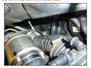
7. Loosen the hose clamp that secures the factory intake hose to the turbo inlet and then remove the intake hose from the vehicle.
