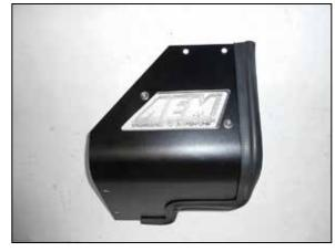
15. Install the remaining 18.75" section of the edge trim onto the heat shield as shown.
