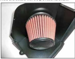
13. Install the air filter onto the adapter and secure with the provided hose clamp.
