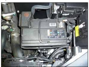
20. Slide the battery back into position and secure with the factory hardware.
