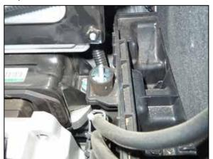
18. Install the provided rubber mounted stud onto the factory air filter housing mounting location as shown.
