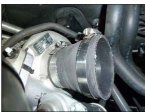
8. Install the provided coupling hose (08188) onto the turbo inlet and secure with the provided hose clamp.
