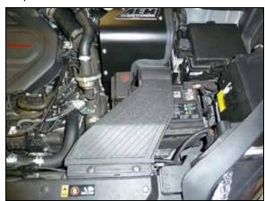
24. Reinstall the fresh air intake duct and secure with the factory retaining pins.
