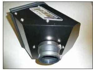
17. Install the provided coupler (084055) onto the filter adapter and secure with the provided hose clamp.
