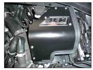
19. Install the AEM® air filter assembly so the mounting studs insert into the mounting grommets and then secure to the rubber mounted stud using the provided hardware.
