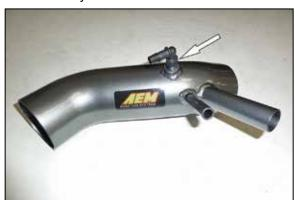
21. Install the provided 90° vent fitting into the AEM® intake tube as shown.
