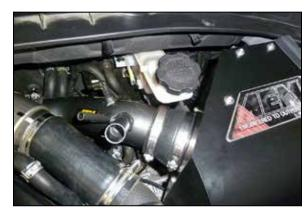
22. Install the AEM® intake tube into the couplers, align the tube for best fit and then secure with the provided hose clamps.
