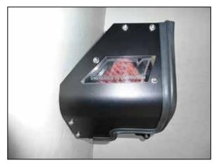
16. Install the lid onto the heat shield and secure with the provided hardware.
