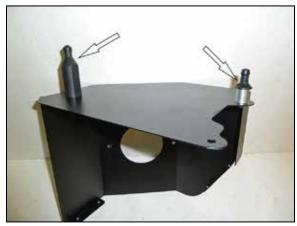
11. Install the two provided mounting studs onto the heat shield.
