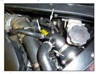
23. Connect the 3 vent lines to the fittings in the intake tube and secure with the factory spring
