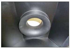
12. Install the provided filter adapter into the heat shield and secure with the provided hardware.
