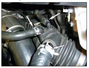
6. Release the spring clamps that secure the vent lines to the factory intake hose and then disconnect the vent lines from the intake hose.
