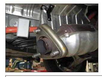
f. Install the supplied gasket (RM-CB84) on the OEM catalytic converter as shown.
