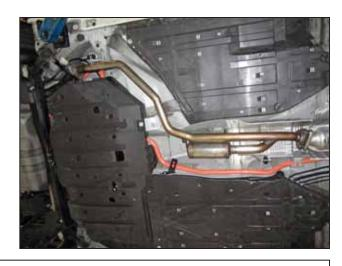
g. Install the AEM $^{\rm @}$  mid pipe (83034) as shown by engaging the two rubber mounts.
