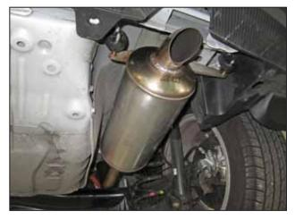
c. Install the rear section of the AEM® exhaust (83035) as shown, by engaging the two rubber mounts at the muffler.
