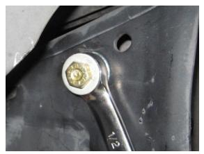
X. While keeping the Threaded Insert flange firm and parallel against the frame rail, tighten the screw using a 7/16" box end wrench or socket. Turn it 2.5 rotations to set the Threaded Insert. Tightening in ¼ turn increments tends to work well.
