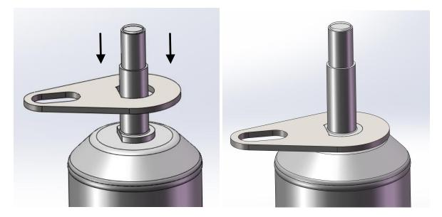
E. Slide the Lower Bushing (BOM item #5) and the appropriate Alignment Washer for your vehicle (BOM item #6 or #7 depending on year; see BOM on page 2) over the threaded pin on the shock body as shown below.
