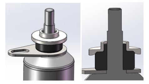
F. Install the lower shock mount and thread in the OE lower shock bolt/washer that was removed in step A. Thread in until the lower shock mount is almost snug, but don't tighten yet.
