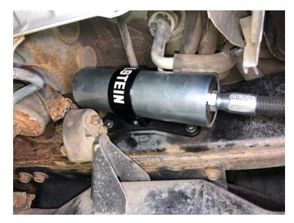
JJ. Once the reservoir has been positioned as shown and confirmed to not be contacting anything on the vehicle, tighten the Socket Head Cap Screw that was snugged down in step HH. **Torque the Socket Head Cap Screw to 6 ft-lb (8 Nm).**
