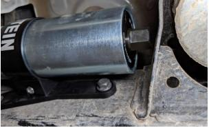
T. Once the reservoir has been positioned as shown and confirmed to not be contacting anything on the vehicle, tighten the Socket Head Cap Screw that was snugged down in step P.
