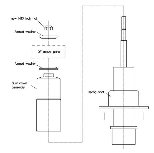
Refer to vehicle service manual for removal and installation of the front shock absorber. Refer to the diagram above for assembly of shock absorber only,
