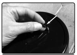
**13.** Place the 3mm vacuum cap on top of the Injen filter if you are not using the optional Filter Monitor Kit P/N AC1000
