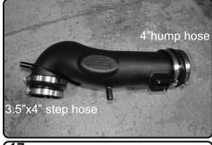
17. Install the 3.5"x4" step hose with clamps to the intake tube. Install the 4" hump hose to the intake tube with clamps. For 6.2L only, use provided 4" straight hose on throttle body.
