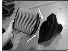
**16.** Install the filter to the plenum, secure and tighten using 8mm nut driver.
