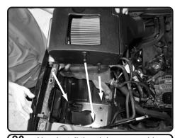
**20.** Now install the air box assembly into the vehicle. Position the tabs to seat like OEM box.
