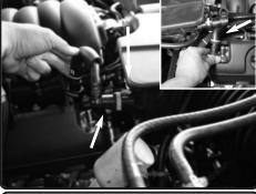
**7.** Disconnect both of the crank case lines from the air box and engine and remove the hard lines from vehicle.
