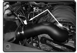
**22.** Install the intake tube. Secure the tube to airbox and throttle body. Position for best fit and tighten clamps. Re-connect the MAF sensor Harness.
