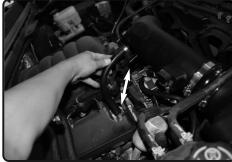
**23.** Install the provided 8.5" 15mm hose to the fitting on engine and intake tube on passenger side.
