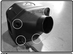
**18.** Now secure the plenum using provided 4 M6 screws and rubberized washers. Secure and tighten.
