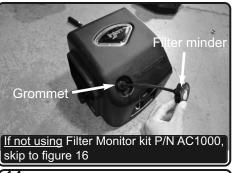
**14.** Install the provided grommet to the hole on air box, now attach the 3mm vacuum line to the filter minder and install the filter minder to the air box. Place hose through the grommet.
