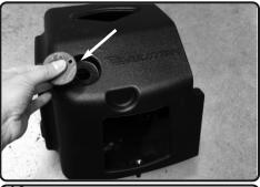
**12.** Push the Filter Monitor Plug into the Filter Monitor pod on the Injen air box if you are not using the Filter Monitor Kit P/N AC1000
