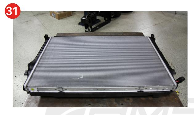
**32.** Install the AMS intercooler in the reverse order making sure the upper mounting clips are fully seated.
