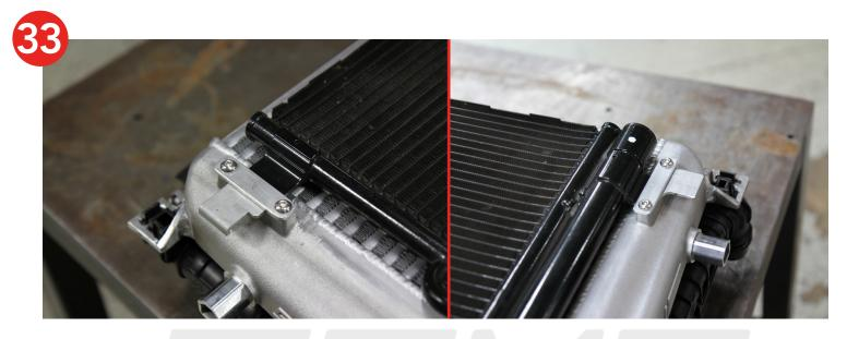
**34.** Reinstall the cooler assembly retaining clips. Replace is necessary.
