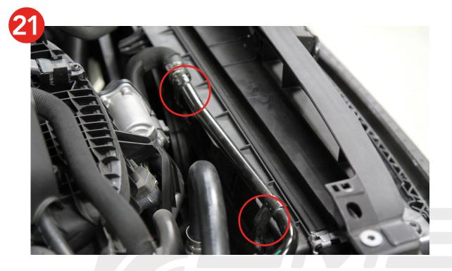
22. Disconnect both horn connectors and harnesses. The horns can remain bolted into place.
