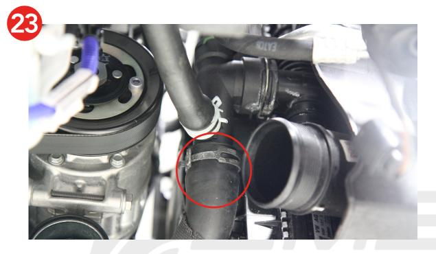
**24.** When the coolant is drained, reinstall the radiator hose. Disconnect both main radiator hose connections at the radiator quick connects by sliding out the metal retaining clip.
