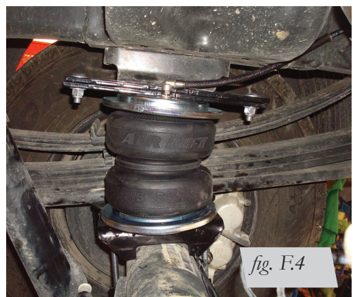
Inside view of the passenger's side installation.
