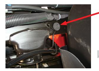
Remove the bolt and discard the wire retaining bracket
