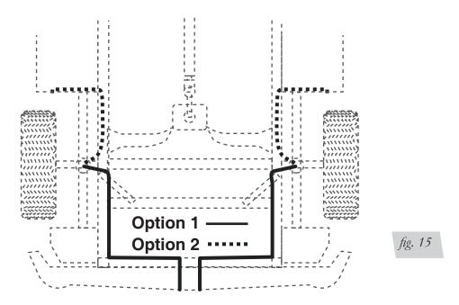
7. Cut off the air line, leaving approximately 12" of extra air line. A clean square cut will ensure against leaks. Insert the air line into the air fitting. This is a push-to-connect fitting. Simply push the air line into the 90° swivel fitting until it bottoms out (9/16" of air line should be in the fitting).
