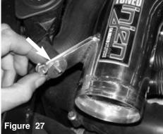
The fender washer and m6 flange nut is placed over the secondary intake vibra-mount stud as shown above.
