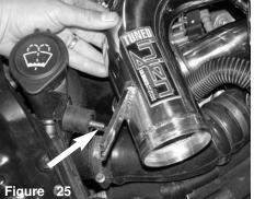
As the intake is inserted into the turbo inlet, the intake bracket is aligned to the vibra-mount stud.
