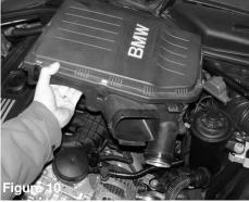
Once the air box has cleared the brake line, continue to pull the air box out of the engine compartment.
