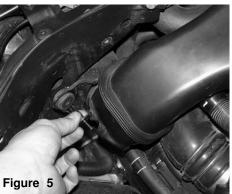
Loosen and remove the 10mm bolt that secures the air duct in place.
