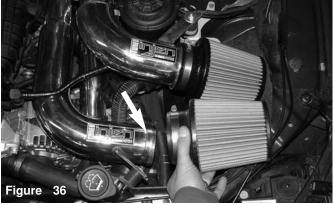
The secondary filer is now aligned to the secondary intake as shown above.
