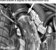
The secondary intake is aligned to the rear turbo inlet. As the intake is inserted into the turbo inlet, the intake bracket is aligned to the vibra-mount stud.
