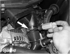
The front turbo inlet clamp is loosened from the air box cleaner.
