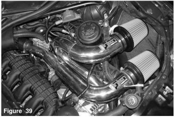
Periodically, check the fitment of both intake systems. Normal driving conditions may loosen nuts, bolts and clamps causing intakes to shift resulting in damage to automotive parts.
