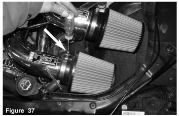
Once the filter stops are butted up against the intake end, continue to tighten the filter neck clamp.
