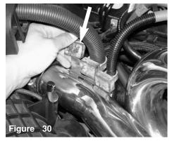
The rubber harness supports are aligned and pressed over the aluminum prongs>
