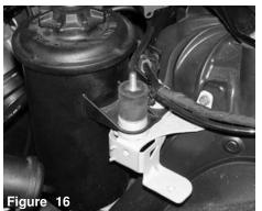
The male/female vibra-mount is fully fastened over the stock vibration mount.
