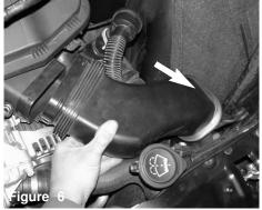
The air scoop is detached from the air box cleaner and pulled out of the engine compartment.
