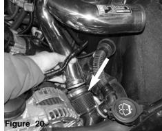
The primary intake is lowered into the engine compartment. As the intake is aligned to the turbo inlet, the intake bracket is aligned to the vibra-mount stud.
