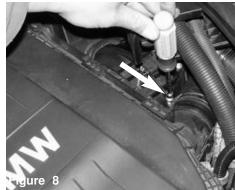
The rear turbo inlet clamp is loosened from the air box cleaner
