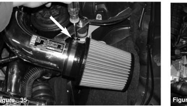
Use a 10mm press nut to fasten the filter neck clamp.
