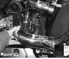
The secondary intake is now lowered into the engine compartment. The intake is aligned and pressed into the rear turbo inlet.
