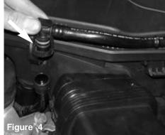
The brake vacuum line is removed
