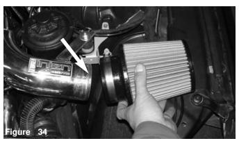
The filter is now aligned to the primary intake. Once the filter stops are butted up against the intake end, continue to tighten the filter neck clamp.
