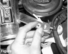
The m6 flange nut and fender washer are placed over the primary intake bracket as shown above.
