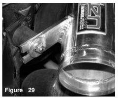
The secondary intake is now secured to the vibramount stud
