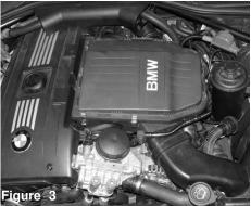
Stock air intake cleaner and air ducts shown in this
