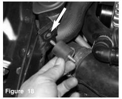
The m6 vibra-mount is aligned and screwed into the radiator brace.
