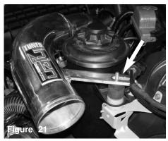
The intake bracket is aligned to the male/female vibramount as shown above. The m6 flange nut and fender washer are installed later in the instructions.
