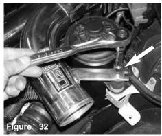
A 10mm socket or nut driver is used to fasten the flange nut to the m6 vibra-mount.
