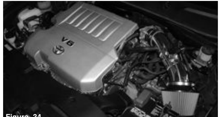
Figure 34 Congratulations! You have just completed the installation of this intake system. Periodically, check the alignment of the intake, normal wear and tear can cause nuts and bolts to come loose. Failure to check the alignment and adjust the intake can cause damage that will void the warranty.
