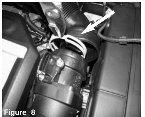
Figure 8 With pliers, carefully pinch clamp and pull intake tube away from air box.
