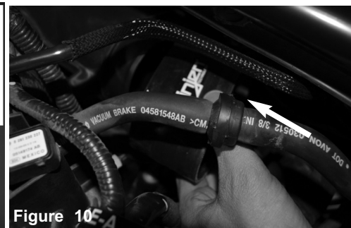
Figure 10 Install the 3-1/2" hose to the oval intake tube plenum.
