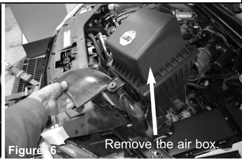
Figure 6 Lift up and remove factory air box assembly.
