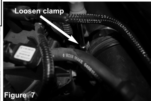
Figure 7 Loosen the clamp on the intake tube plenum. This is where the new intake system will attach.
