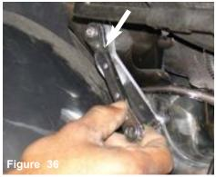
A ratchet or nut driver is used to fasten the m6 flange
