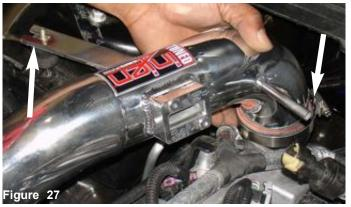
Once you have aligned the intake bracket to the vibra-mount , continue to press the intake into the hose over the throttle body.  $\frac{1}{2} \int_{-\infty}^{\infty} \frac{1}{2} \left( \frac{1}{2} \int_{-\infty}^{\infty} \frac{1}{$
