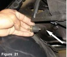
The male vibra-mount is inserted into the pre-drilled hole located on the passenger side bumper support.
