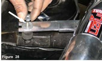
The m6 flange nut and washer are used to fasten the intake bracket to the vibra-mount stud.
