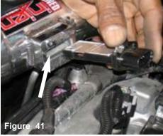
The mass air flow sensor is slowly lowered into the machined sensor adapter.
