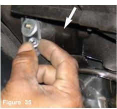
The new filter is aligned to the end of the intake and pressed over the intake.
