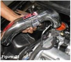
The primary intake is now lowered into the engine compartment.
