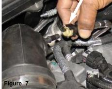
The vacuum port connector is removed from the air duct port as shown above.
