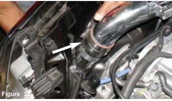
As the secondary intake is inserted into the corner bumper, the top end is aligned to the silicone hose. The intake bracket is also aligned to the vibra-mount stud.
