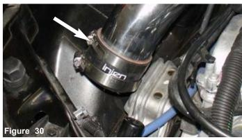
The silicone hose is pressed over the end of the primary intake, a power band is used to secure the silicone hose over the intake end.
