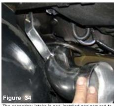
The secondary intake is now installed and secured to the vibra-mount.
