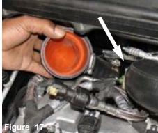
The silicone elbow is now lowered into the engine compartment and over the turbo inlet. The clamp over the turbo is now semi-tightened.
