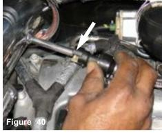
The vacuum clip is pressed over the machined vacuum port.
