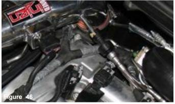
Check the harness clip and vacuum lines for proper fitment. Make sure there is good contact between the harness clip and mass air flow sensor, check for any possible vacuum leaks in the vacuum connections.
