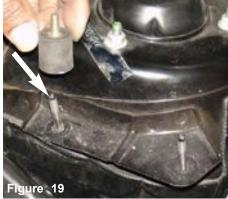
The male/female vibra-mount is aligned and screwed over the air box stud.
