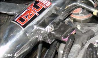
The mass air flow sensor and electrical harness clip are now installed.
