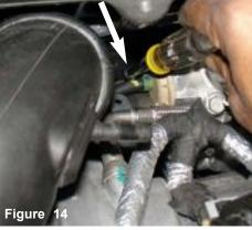
The lower turbo air inlet clamp is now loosened as shown above.
