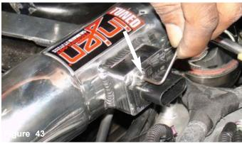
An allen wrench is used to fastened the m4 bolts to the machined adapter.
