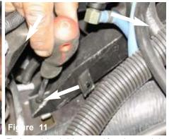
The lower air box bolt is removed from the extended brace.
