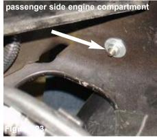
The m6 flange nut is placed over the vibra-mount stud located on the opposite side of the fender or inside of the engine compartment.
