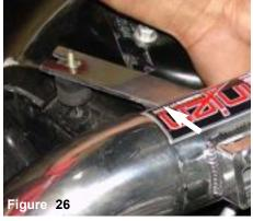
As the primary intake is aligned to the turbo inlet, the intake bracket is aligned to the male/female stud.
