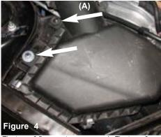
The two m6 flange nuts are removed. The top m6 flange nut has already been removed (A)
