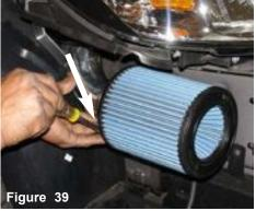
Once the filter is sitting flush over the intake end, continue to tighten the filter clamp.
