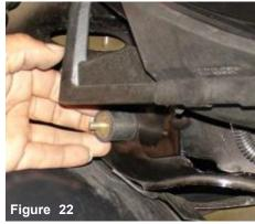
The vibra-mount is inserted into the bumper support frame. The nut and washer is lowered from the inside.
