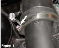
The turbo air inlet clamp is loosened in order to separate the air box from the air intake duct.
