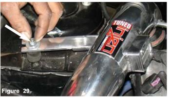
The m6 flange nut is tightened.
