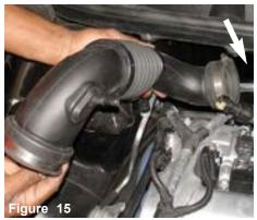
The lower air duct is now pulled out from the engine compartment.
