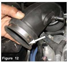
The turbo air inlet duct is disconnected from the air box cleaner
