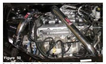
Periodically, check the fitment of both intake systems. Normal driving conditions may loosen nuts, bolts and clamps causing intakes to shift resulting in damage to automotive parts.
