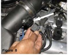
The tab is depress and the electrical sensor harness is removed from the mass air flow sensor.
