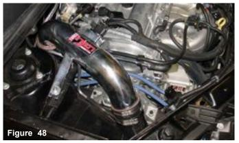
Check the connection of the intake bracket to the vibra-mount and the alignment of the primary and secondary intakes. Everything should be properly aligned to prevent damage to the cold air intake.
