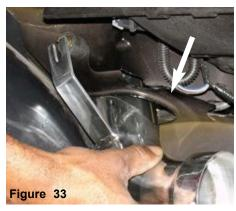
Once you have aligned the secondary intake to the vibra-mount, continue to tighten the m6 nut.
