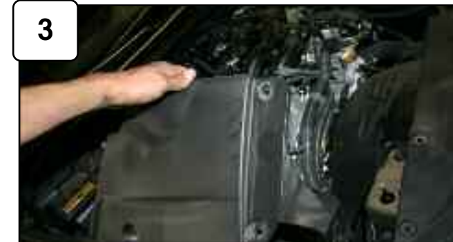
Remove engine cover and front/passenger plastic covers.
