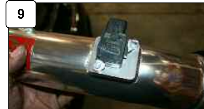
With provided M4 screws, install MAF sensor to new intake tube.
