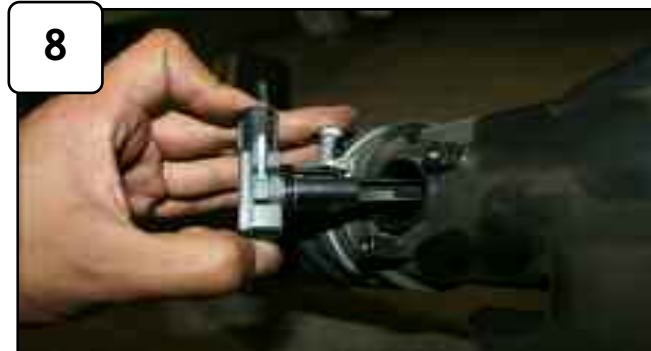
Remove MAF sensor using phillips screwdriver.
