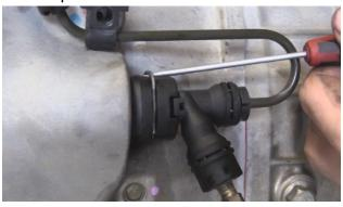
4) Pull the hard line out of the slave cylinder.
