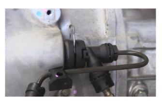
3) Use a flat blade screwdriver to pop the retaining clip up and remove it.
