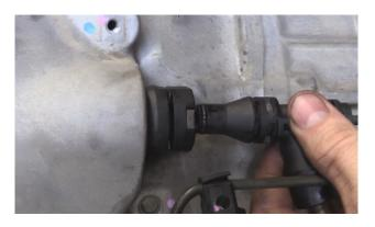
5) Inside the bellhousing remove the M6 bolt that supports the CSC pipe, along with the 3 bolts that mount the CSC to the gearbox.
