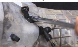
2) Rotate the clutch line down toward the bleeder
