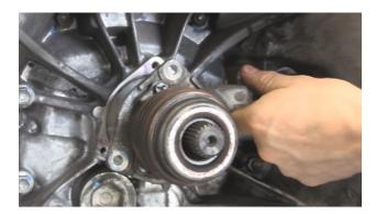
6) Thoroughly clean the bellhousing of old clutch dust and grease and ensure that the CSC mounting surface is free from any debris or burrs, to ensure that the new CSC spacer sits flush.
