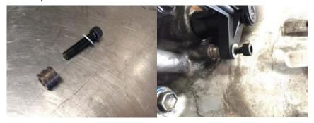
3) Clip the old hard line into place on the new CSC. Flip the line back up into place and re-install the bolt to support this line on the bellhousing.
