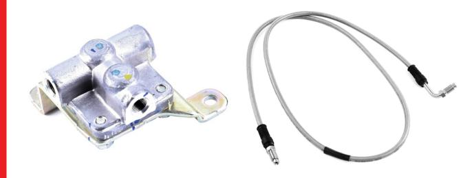
Installing this line will increase the pedal feel and give a more positive clutch engagement.
