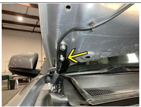
4. Remove the rear hood hinge bolt. Carefully rotate the bracket so that the rear ditch light bracket hole lines up with the rear hood hinge mounting hole. Secure the bracket with the provided M8 bolt and washer by hand tightening the bolt.
