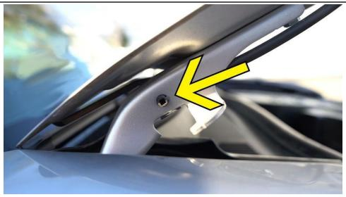
1. Open the hood. On the passenger side hood hinge, use pliers to squeeze the two tabs of the plastic clip to detach the washer fluid hose from the hinge.
