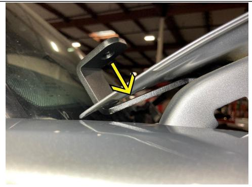
5. The ditch light brackets have slotted mounting holes to adjust for clearance. When aligning the bracket, the hood hinges, and the hood, make sure everything is aligned correctly.
