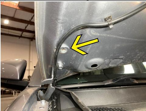
2. Remove the top bolt from the hood hinge as shown in the image above.
