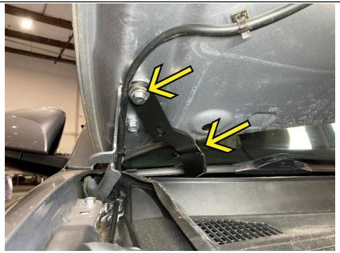
3. Install the right ditch light bracket using the provided M8 bolt and washer by hand tightening the bolt. Angle the bracket to provide clearance to remove the rear hood hinge bolt in the next step.
