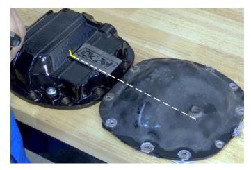
9. Lay the dipstick atop the cover so that it is situated at its final installed depth. Use a scratch awl, needle file or other suitable tool to etch a "full" mark on the dipstick. Install O-ring on dip stick, and install dip stick in cover.
