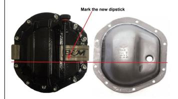
9. Apply a bead of RTV silicone gasket maker to the B&M Cast Iron Diff Cover. Run the bead inside the bolt holes. If your vehicle has a reusable gasket it may be reused but check the condition of it.
