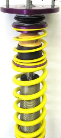
Tightening torque for the top fitting is 25 Nm (18 ft-lb). Please install the strut unit to manufacturers recommended settings regarding tightening torque and fixing specifications.
