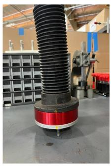
16. Once more compress the coil spring, then tighten the Shock Absorber Top Shaft nut, (in-line) with your markings of alignment, to 88 LB-FT. Finally, unload the spring and remove the Shock Absorber assembly (from the Spring Compressor). Install the Leveling Kit Top spacer, between the Shock Absorber assembly and the vehicle frame.
