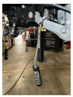
5. Using a Panel Popper tool disconnect and remove shock sensors by pulling and pushing the tab inward to disconnect.
