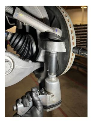
7. Using a 21mm impact socket, remove the Sway Bar End Link nut, and proceed to remove the lower sway bar link joint from the lower control arm.
