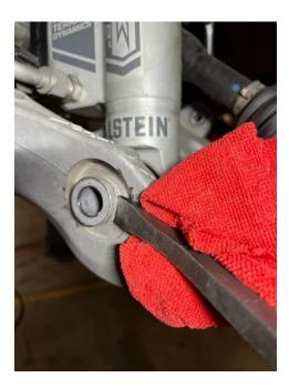
11. Remove the Upper Control Arm Ball Joint nut, and separate the Upper Control Arm from the steering knuckle, pop the wire clips from the top of the shock studs, and remove the Upper Shock Absorber Stud nuts using a 16mm wrench. Finally, remove the Shock Absorber assembly from the vehicle.
