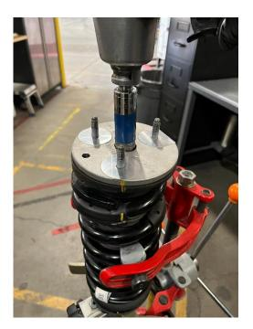
14. Remove the Shaft Boot and cut the lip off at the designate location.
